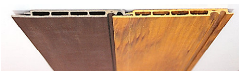
"EAZY-CEIL 8121" 8 thk. x 121 x 3,050 mm (T&G with ~4mm groove width)
